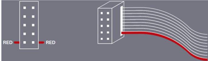
If you flip over your VCV RANDOM, you will find the "RED" mark at the PCB power connector, which must match the colored line on the ribbon cable. Once you have checked all the connections, you can turn on your modular system. If you notice any anomalies, turn your system off right away and check again your connections.
