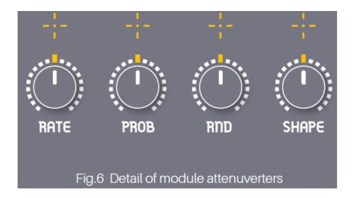
In the center position (0), the signal does not affect the parameter. If you turn it to the right, it attenuates (turns down the strength) the signal. If you turn it to the left, it inverts the signal, making things that were going up, go down instead, and vice versa.
