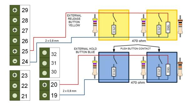
The NANO has a separate input for external extinguishing release and external hold off button.
