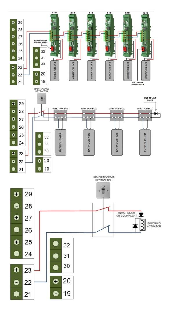
A connection as shown with a junction box is technically possible. But it is not covered by our warranty. We can only guarantee the proper functioning of the NANO in combination with an ETB. Only an ETB has a bridge protection against a possible early blockage, which ensures that the activation current flows through all igniters at all times.
