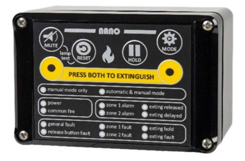
The NANO/MAR control panel should be mounted on a dry, flat surface, at eye height in a horizontal position so that the enclosure cannot deformed. The NANO/NAO should be installed in an accessible area. The enclosure is provided of 7 predrilled holes for M16 cable glands. Enclosure material is ABS suitable for outdoor use IP65. To ensure the IP rating the cables must be brought in using appropriate cable glands. Dimensions enclosure 120 x 80 x 58.5 mm w x h x d
