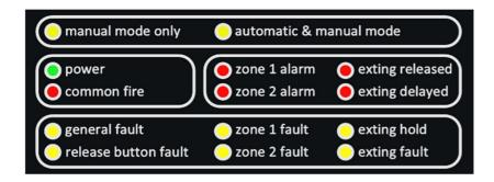
The NANO has 3 internal and 14 front LED indicators. Under normal condition only the green Power LED and either the Manual Only or Automatic and Manual LED lite.
