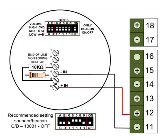
By a single sounder beacon follow the connection diagram below. The recommended setting gives the best and deviating alarm signal compared to the usual evacuation alarm signal for example on vessels. In some cases, the installation of a second signaling device is necessary. For more options, and wiring advice, please refer to our comprehensive user manual.
