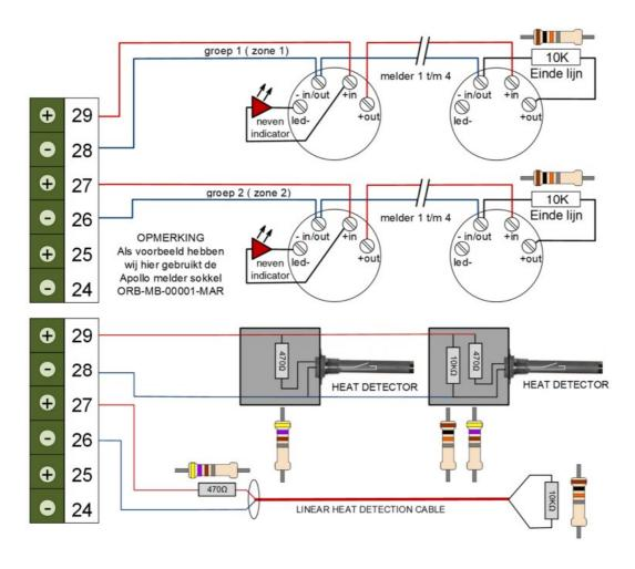
There are 3 options for connecting fire detectors to the NANO alarm panel.
