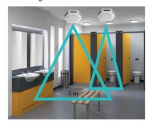
Sensor covers  $\sim$ 2 – 2.5 meter radius zone. Best sensor mounting height is up to 3 – 3.5 meters.
