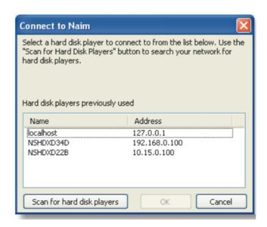
If the HDX is not immediately listed, check that it is connected to the network and switched on, and click on Scan for hard disk players.
