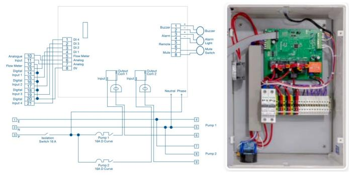
Ensure all floats are connected as normally open (NO) and as an open circuit when the float is in the down position
