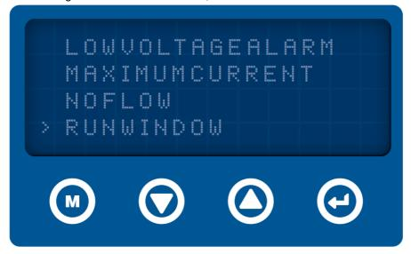
To programme the run window, select Parameters on the LCD screen then scroll down and select Run Window.
