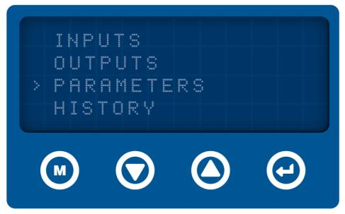
Select Set High/Enable to set the overload current using the up and down arrows. Press Enter to accept the new value or M to exit the screen without changing it.
