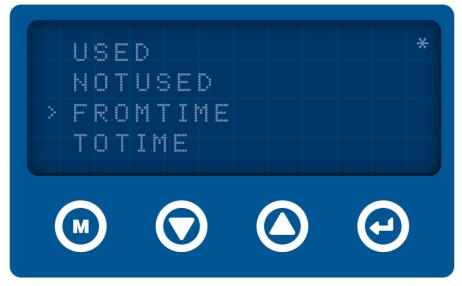
In this screen, select Used by moving the cursor to Used and pressing the Enter Key.
