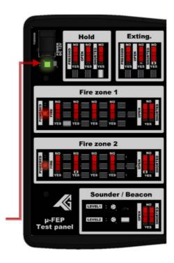
These resistors are also present on the FTM test module. All possible alarms and faults can be simulated by using the switches.
