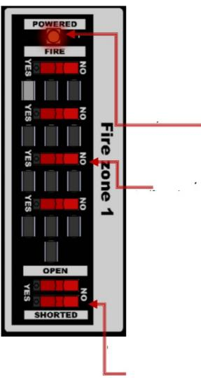
A fire alarm for each fire detector in each fire alarm zone can be simulated by setting the red switch into the YES position. A fire indication in 8fire alarm zone 19 on the NANO is the result. The red common FIRE LED lit and the red fire zone LED lit.
