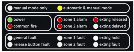
On the FTM 5 clear extinguisher igniter LEDs flash frequent on the FTM panel. This signal confirms a successful activation. It does not work when power is supplied via a laptop connection and/or the emergency power battery, but only and exclusively when used with the included switch mode power supply.
