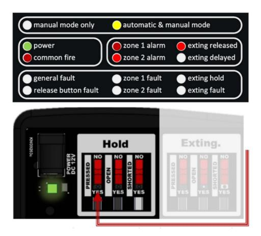
In the event of a fire alarm in both fire alarm zones or when operate the EXTING switch in the YES position, and an extinguishing release delay is programmed, the red 8delay9 LED lite. When operating the HOLD switch, the tone signal will change, and the yellow 8hold9 LED is lit in the 8Extinguishing9 group. This operation does not apply when DIP switches 6 & 7 and 8 are programmed. Refer to the NANO manual for this.
