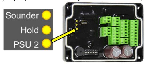
If a standby power source is not available, then the connection points 17/18 must be connected to respectively point 14/15 to avoid an fault message.
