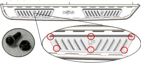
**Step 3:** Install the supplied rocker panel brackets (x6) to the attachments points located on the backside of the main tube (Driver/Passg) using the supplied 3/8" x 1" carriage bolts and 3/8" flanged nuts. Leave finger tight for now.
