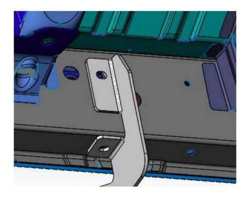
**Step 8:** There will be  $\frac{1}{2}$ " of adjustment in the (x3) mounting bracket. Adjust to desired position and tighten to (20 ft,/lbs).
