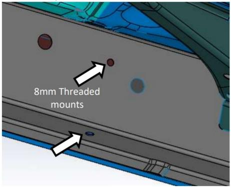
**Step 5:** Carefully raise the Nerf Board assembly up into position aligning the mounting brackets with the factory-threaded holes. Beginning with the center bracket start one of the supplied M8x30mm Hex bolts in the upper mount and finger tighten. This will allow the step to suspend while you start the reminder of the hardware.
