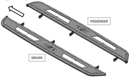
**Step2:** Install the supplied step plate (x2) to each Running Board using the M6x20mm button head bolts, M6 nuts and M6 flat washer.
