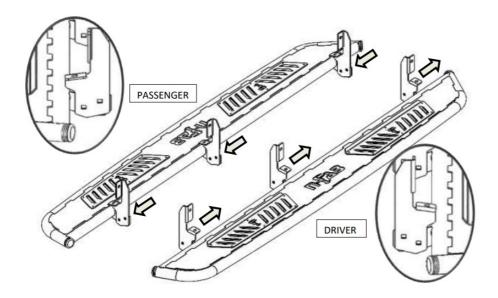
**Step 4:** Remove factory-running bards (Both sides) if equipped and discard. You will see the 8mm threaded mounts in the body.
