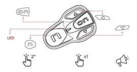
Press and hold the button for the number of seconds indicated. Press and release the button for the number of times indicated. Voice prompt.
