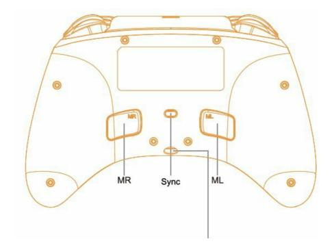
3.5mm jack(only when the controller connects to console via cable)
