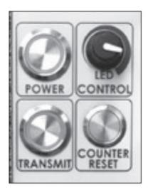
TRANSMIT Generates 512hz signal at camera head for use with a Locator. This has nothing to do with Wi-Fi transmission.
