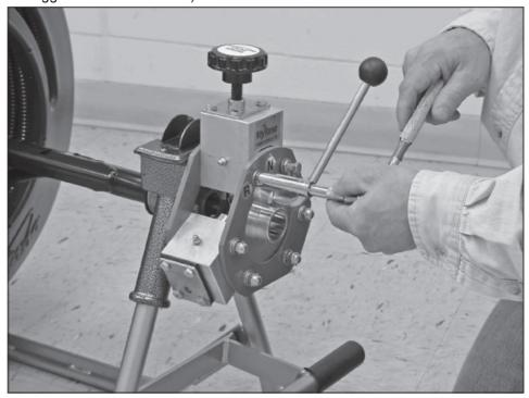
**Step 3**Secure the Autofeed into place by threading the bolts into the holes.
