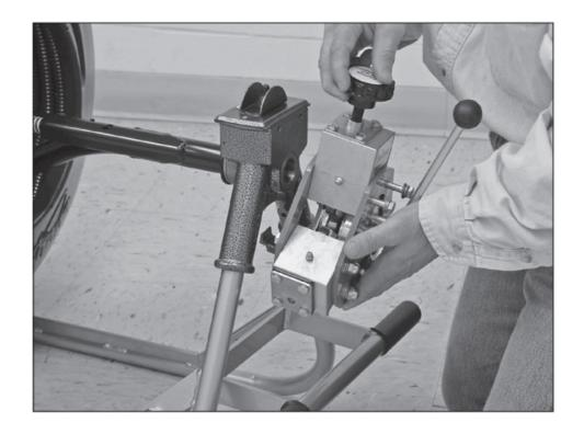
**Step 1**Pull the top two bolts (that hold the top cylinder in place) back flush with the backplate of the Autofeed. **Step 2**
