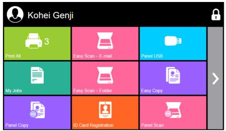
The action nodes correspond to buttons on the printing device display. On the MyQ Web administrator interface, you can configure the layout of the display screen, as well as the behavior of each button. Therefore, you are free to choose any combination of available actions and their positions on the screen. The layout is displayed on a WYSIWYG (What You See Is What You Get) terminal preview and can be configured there.
