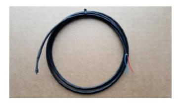
If the sensor (see figure) indicates a value >80 °C the pins may not be connected correctly or there might be a sensor break. A negative value can be an indication of a short circuit.
