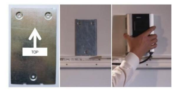
To fix it to the wall bracket, the AC • THOR is suspended in the wall bracket by the two long slots on top and then fixed in place by locking it underneath (slide to the left).
