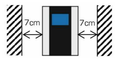
When installing several devices side by side, a minimum distance of 10 cm must be observed!
