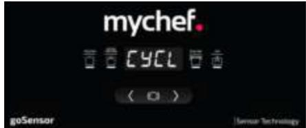
To stop showing this value and to finalize the appliance start-up process, press the centre button again. Once the vacuum packer is connected to the electricity grid and the start-up process is finalized (whether the pump status values are checked or not), the appliance will turn itself off. The user is required to turn the appliance on in order to begin operating.
