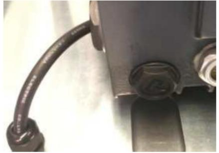
Place a container below the hole for the oil to drain into, in order to keep the vacuum packer shelf clean.
