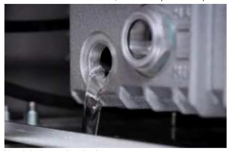
When all of the oil has drained out, replace the plug.
