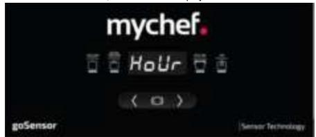
Pressing the centre button while the number of pump operating hours is being displayed will show the number of vacuum cycles completed by the vacuum packer. The value will be displayed in the same way as above, but instead of "Hour" indicating the end of the number of operating hours, the screen will show "Cycle" to represent the vacuum packing cycles.
