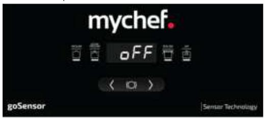
• In this mode the vacuum packer will turn off automatically after a few seconds. If you wish to turn it off immediately, you will need to press the centre button.
