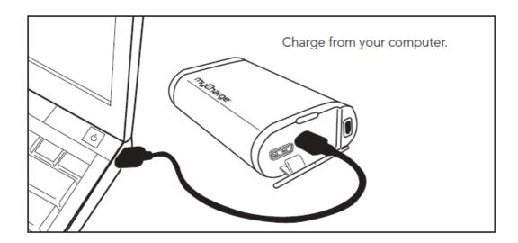
Connect the included charging cable with the Micro-USB tip through your computer's USB port or a USB AC power adapter. Times to charge the Universal Charger 6000 vary based on what it's plugged into. You can expect a full charge from a USB AC power adapter in about 7.5 hours or from a standard USB port in about 13.5 hours.
