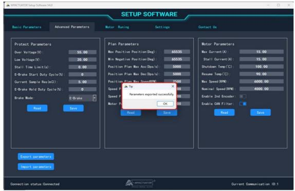
After exporting the parameters successfully, you can find thexxx file storing the parameters in the specified path and open it to see all parameters.
