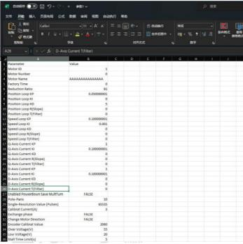
It is not recommended to modify the contents of the xls file, which may cause errors in the import parameters.
