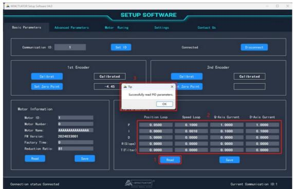
Click the "Save" button of PID parameter, it saves all PID parameters to the motor program, and the pop-up window prompts "Successfully saved PID parameters.", as shown in Figure 2-9. To prevent operational errors, as long as there is no value for any parameter, the setup software will not perform any operation when clicking the "Save" button.
