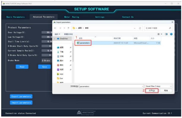
The setup software will read all parameters in the file, write all parameters to the motor, and pop-up window prompt "Parameters were imported to the motor successfully.
