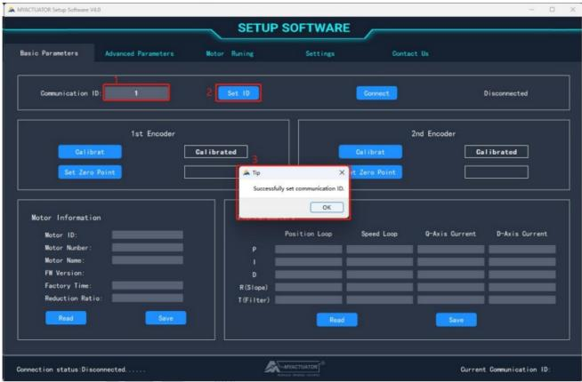
Click on the "Connect" button to connect successfully, then this button can not be used, and display "Connected", display encoder calibration, the current position, motor information, and the current communication ID.
