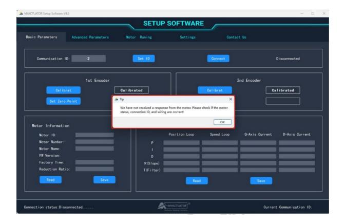
Troubleshooting the failure to respond received from the motor.
