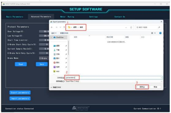
The software will read all parameters in the motor, in the specified path to the specified file name to create an xix file, write all parameters to this file, and pop-up window prompts "Parameters exported successfully."
