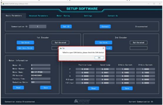
Troubleshooting the failure to open the CAN device.
