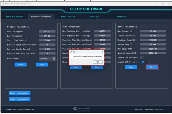
To prevent operational errors, the setup software does not perform any operation when the "Save" button is clicked as long as there is no value for any of the motor parameters.
