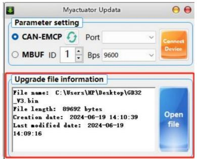
Click the "Update" button, for motors with the operating program, the setup software can directly write the upgrade firmware into the motor without re-powering. After successful download, as shown in Figure 6-3, you can directly close the update software.
