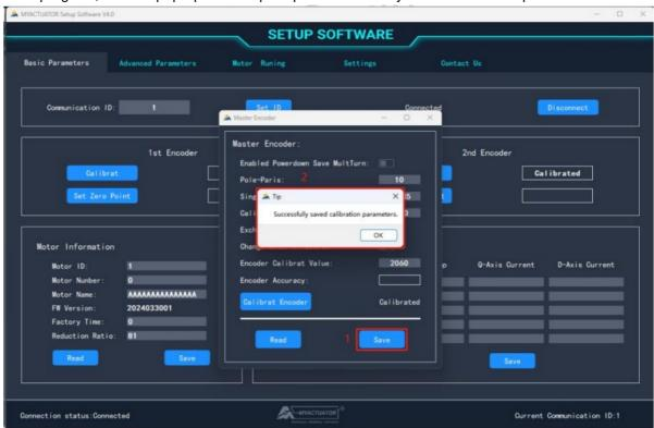
Prevent operational errors, as long as there is no value for any one parameter, click the "Save" button, and the setup software will not perform any operation. Further, click on the "Zero Calibration" button, and you can control the motor calibration.
