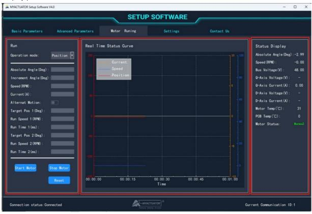
The motor can be controlled to run in a certain mode. Click the "Stop Motor" button to stop the motor. In addition, when switching to the basic parameter screen and advanced parameter screen, the control motor is stopped to prevent accidents. Click the "Reset button to restart the motor master controller. The real-time status curve part collects data in real-time and draws dynamic line graphs, so you can view the curve changes within one minute, and the specific meaning of the line.
