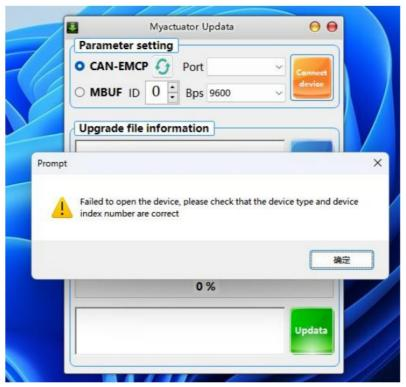
Troubleshooting the failure to open the CAN device.
