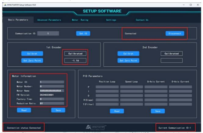
Click on the "Disconnect" button, operate the setup software to close the CAN-USB conversion device, then display "Disconnected", and the connection status changes to "Not connected...", and the current communication ID is cleared.
