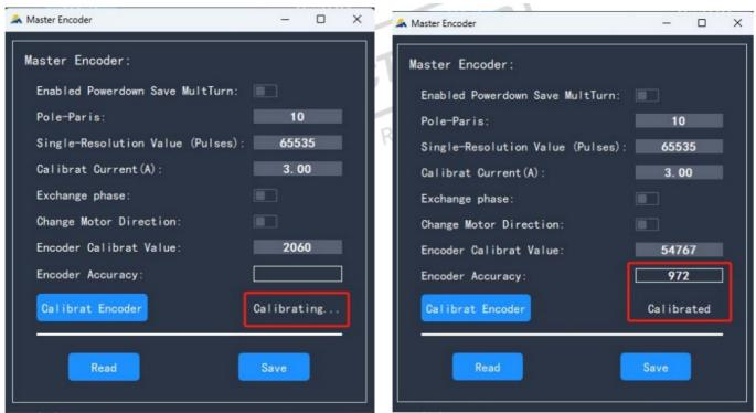
After calibration, re-read all data in the "Master Encoder" interface and display the calibration result. If the calibration is unsuccessful, the resolution is shown in Table 2-3. In addition, some motors will automatically open the "Exchange phase" option after calibration, which is a normal phenomenon.
