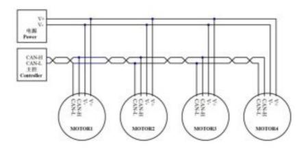
Note: Both ends of the bus need to be connected to 120-ohm terminal resistance
