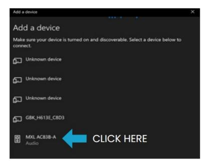
The PC and microphone will now attempt to establish a Bluetooth connection. Once the device has been successfully paired, the flashing on the MXL AC83 will stop and the yellow LED will remain illuminated. A message will pop up on screen indicating that the pairing was successful.
