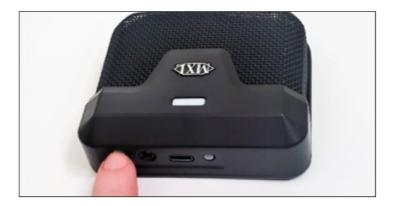
The blue and yellow LEDs will begin flashing to indicate that the unit is in pairing mode. MXL AC83-A should now appear in the Bluetooth menu. Click the Connect button to initiate a Bluetooth connection.
