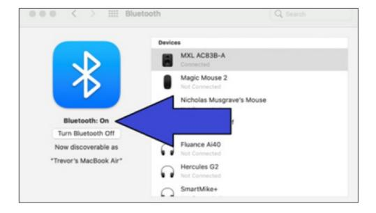
Next you will want to initiate pairing mode on the MXL AC83. Press and hold the Bluetooth Power Button for 6-8 seconds to enable pairing mode.
