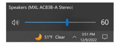
For high quality stereo output with no microphone input, select Speakers (MXL AC83 Stereo) For mono output with simultaneous microphone input, select Headset Earphone (MXL AC83-A Hands-Free AG Audio).
