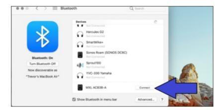
The computer and microphone will now attempt to establish a Bluetooth connection. Once the device has been successfully paired, the flashing on the MXL AC83 will stop and the yellow LED will remain illuminated. Now that a microphone has been successfully paired with the computer, you will need to select the correct sound set-tings. Return to the System Preferences panel and select the Sound icon.
