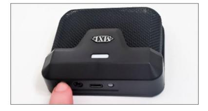
The blue and yellow LEDs will begin flashing to indicate that the unit is in pairing mode. Next click on the Bluetooth option in the Add a device window.
