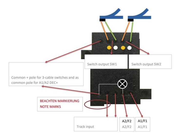
Switch lamps between A1/A2 and common + pole. Use with 3-wire switches the common DEC+ pole as the center line. Not use 3 pole LGB drives!
