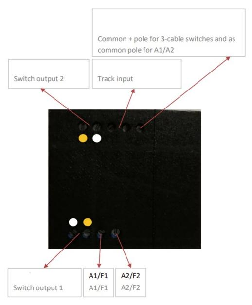
Switch loads between A1/A2 and common + pole. Use with 3-wire switches the common + pole as the center line. Not use 3 pole LGB drives!
