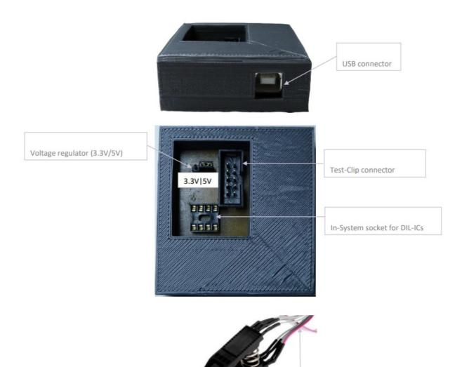
Test Clip; Pin 1 (When SMD-IC in the top left, left side. As seen from above IC has there a notch / hole depression and possibly the side of the chip there beveled).
