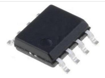
The IC shown above can in contaced circuits via test-clip are. Not all ICs have the hole and yet at the same time the beveled side; at least one marking is, however, always present. The pin directly on top the hole, pin 1; just as in the flattened side (located from above it always looked to the left) is the pin 1 is always at the top left. On the side of pin 1 marked in the test-clip wire to be set.
