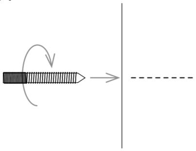
3. Screw on your Dot (be careful not to tighten too hard to avoid damage inside.)
