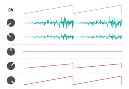
With no CV patched into an input, the attenurandomizer controls the amount of randomization from an **independent internal random source** with a peaky (12 o'clock to fully CCW) or uniform (12 o'clock to fully CW) distribution. The random values from the peaky distribution are clustered towards the middle, with extreme values being infrequently generated.
