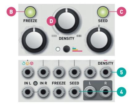
In this mode, the grains are generated continuously, at a rate set by the **DENSITY** knob [**D**] and modulated by the **DENSITY** CV input (5).
