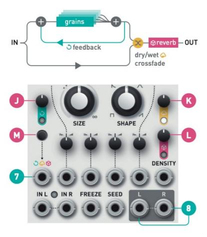
**J. Feedback**, that is to say the amount of output signal mixed with the input signal and fed back into the processing chain. Each quality setting employs a different feedback amplitude limiting scheme typical of the medium it emulates from clean brickwall-limiting to grungy tape saturation.
