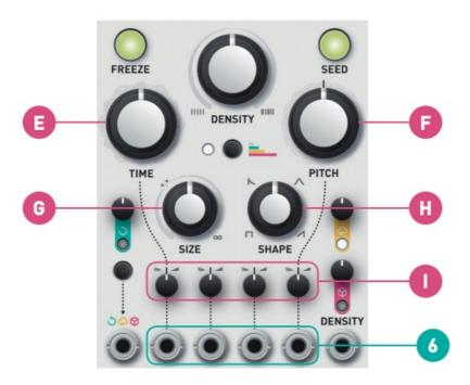
**E. TIME** controls if the grain replays the most recent (fully CCW) or oldest (fully CW) audio material from the recording buffer shifting the replay heads further apart from the record head.
