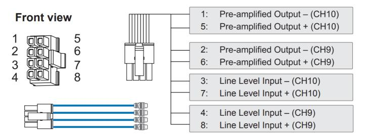
**AUX IN:** Auxiliary low-level stereo signal input to connect an external stereo pre-amplifier source.
