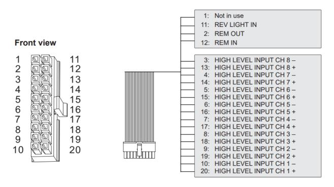
**REV LIGHT IN**: If you connect the reverse gear light cable here, the audio streaming in Bluetooth" Mode will be interrupted and the regular audio from the head unit is audible to perceive signal tones from the park distance control.
