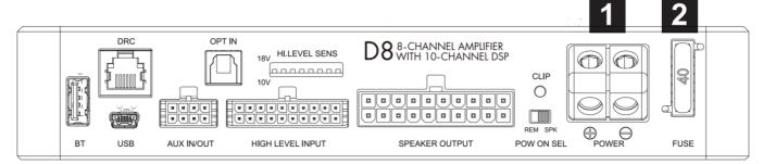
**POWER** Connect the POWER + terminal (+12V) with the +12V pole of the vehicle's battery. Use a suitable cable with a sufficient cross-section (at least 0 5 mm) and install an additional in-line fuse. For safety reasons the distance between the fuse block and the battery should be shorter than 30 cm. Do not set in the fuse into the fuse block until the installation is accomplished.
