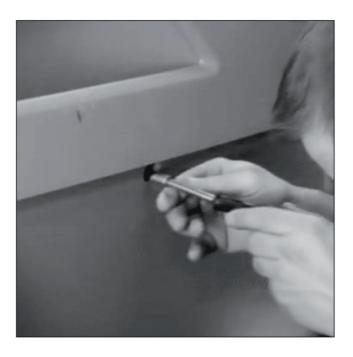
Loosen the screw in the middle of the door panel.
