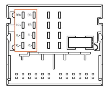
Now connect the speaker cables of the tweeter units with the cables on the back of the Quadlock connector. Please note the assignment of the Quadlock connector on the left.
