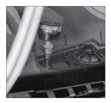
Fasten the new tweeter unit in the installation location with the original screws. Then build everything back again.
