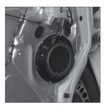
Remove the original speaker. This is riveted six times to the mounting ring. Drill the six rivets and remove them completely from the holes.
