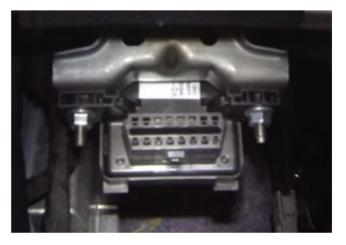
On the back of the DLC module there is a wiring connector that contains the required CAN signals for the CB-2 CAN Interface. The CB-2 should be connected to the DLC module as outlined in the following table.
