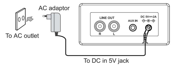
The supplied AC adaptor is suitable for use on AC main supplies of 100-240V AC and should only be connected to the main supply within these parameters.
