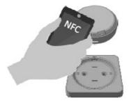
Activate NFC on your phone and tag it on to the bottom of your device. The indicator light will flash red when the device is powered on.
