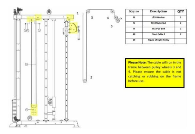
Step 7 – Please note you will have to remove pulley wheels when threading the cable
