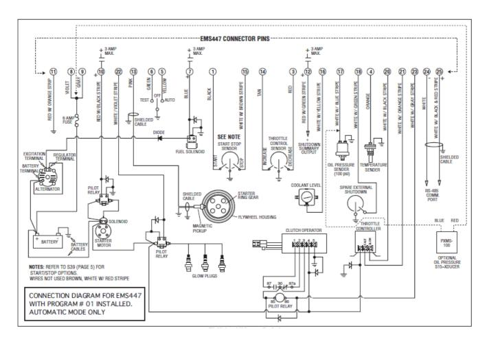
**EMS447 MANUAL MODE Wiring Diagram (S23=Manual)**
