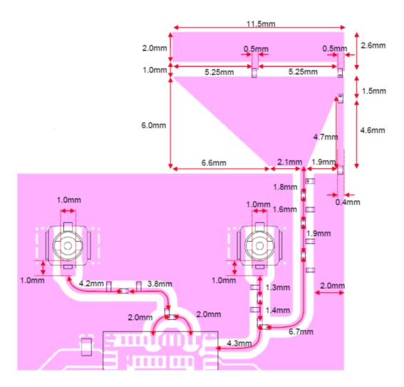
Layout Guidance for Microstrip Design and External Antenna
