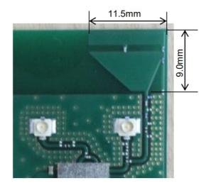
The 50ohm microstrip line and Type2EL\_Antenna needs to be copied when module is installed in the End product.
