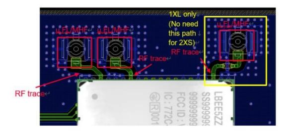
The 50ohm microstrip line needs to be copied when module is installed in the End product. Murata provides set makers with Gerber data or something similar.
