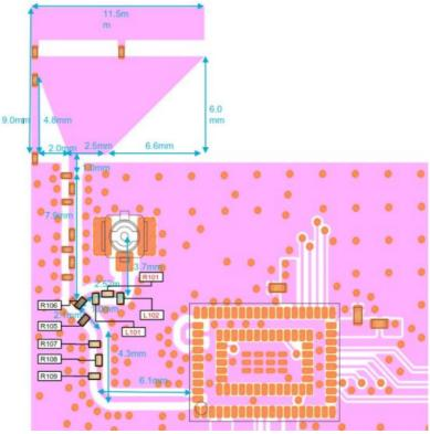
For more detail information, please refer to "P2ML11463\_Type2GF\_For\_DXF.dxf" feed line width: 0.35mm number of substrate layers:  $6 \text{ Substrate thin}: 0.8 \pm 0.1 \text{ mm}$
