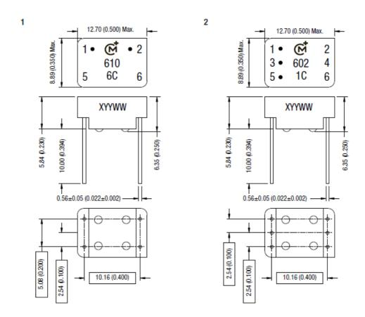
Unless otherwise stated all dimensions in mm (inches)  $\pm 0.25$  (0.01). All pins on a 2.54 (0.1) pitch and within  $\pm 0.25$  (0.01) of true position.
