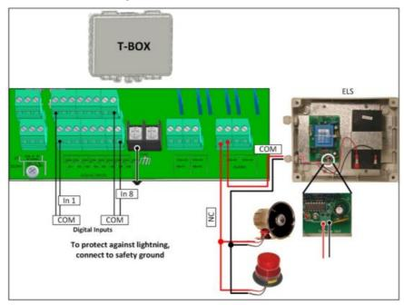
Figure 27: T-Box Wiring Diagram to ELS
