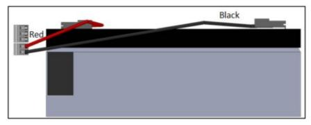
Figure 107: Cable Removal
