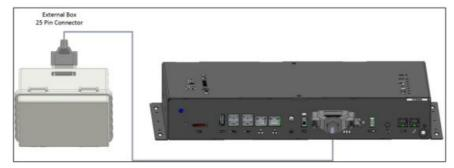
Figure 12: External Box – Communicator 2.0 Plus Cable
