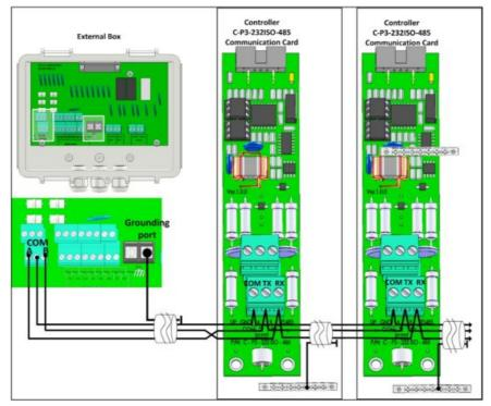
Figure 13: External Box – Controller Isolated RS-232 Connection
