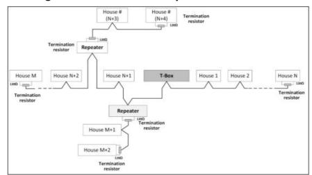
Figure 22: House and Multiple Repeaters Termination
