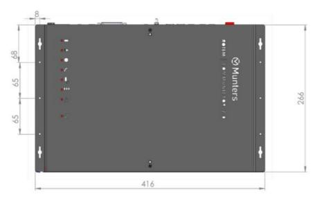
Figure 4: Dimensions (mm)
