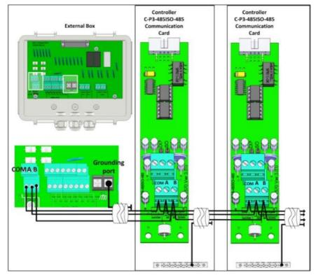
Figure 14: External Box – Controller RS-485 Connection
