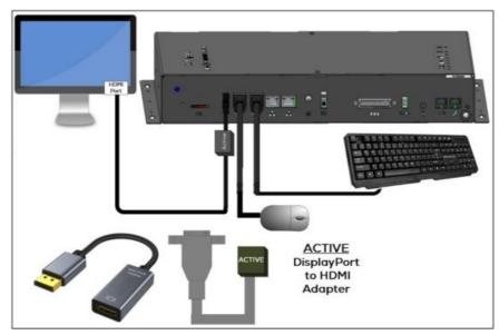
Figure 10: Connection to Peripherals (HDMI to DP port)
