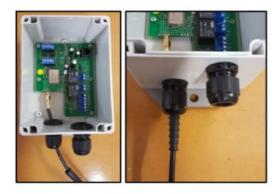
Disassemble the right hand upper cable gland by removing the compression nut, the split rubber insert and the
