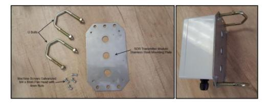
• Install the transmitter module at the top of the mounting pole, approximately 0.5m below the antenna with the cable glands facing downwards. Pass the two U Bolts around the mounting pole and through the transmitter modules mounting bracket. Fit the washers and nuts and tighten the nuts. See the images below.
