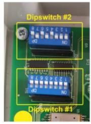
**Dip Switch SW1** is used to set the System ID. This System ID must match the System ID being used by the serial transmitter module in the same control system. The System ID can be set in the range from 0 to 255 using binary. The dip switch numbers conform to the following binary numbers:
