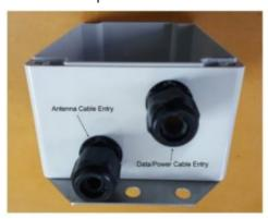
• Feed the antenna cable through the lower cable gland and fasten the SMA connector to the radio board as shown in the images below. Push the protection boot down through the cable gland and tighten the glands compression fitting around the boot to create a water tight connection.
