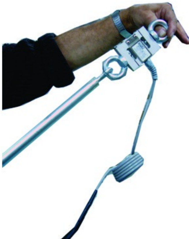
Figure 9: Connect Pole Assembly to Transducer
