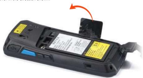
3. Pull on the tab 45° to the upper left, separating the battery from the contacts or terminals inside the device.
