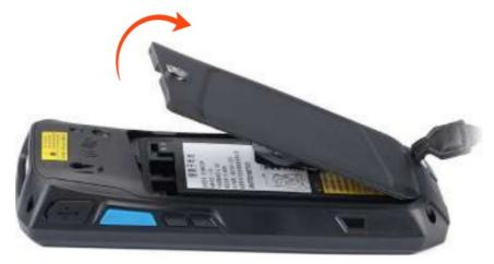
2. Lift the battery cover in the direction shown.
