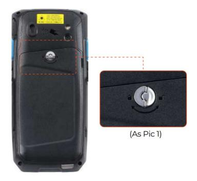
1. Turn the battery cover fastener counterclockwise.
