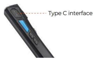
Locate the charging port as shown in the picture, remove the waterproof plug, and charge the device using a USB charging cable that supports the Type-C port.
