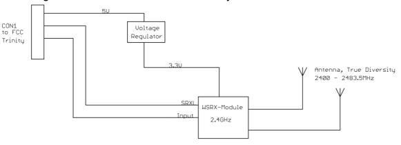
SRXL: Serial RC-Channel Output Input: Telemetry Data
