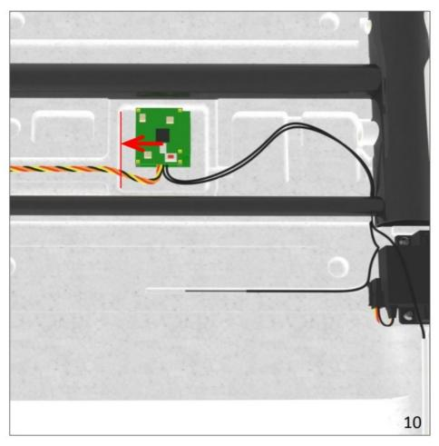
The Two Antenna wires are mounted inside the wing in a 90° angle.
