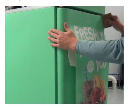
30. With one hand remove remaining backing while guiding the decal onto the panel with other hand.
