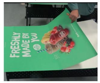
16. With one hand remove remaining backing while guiding the decal onto the panel with other hand.
