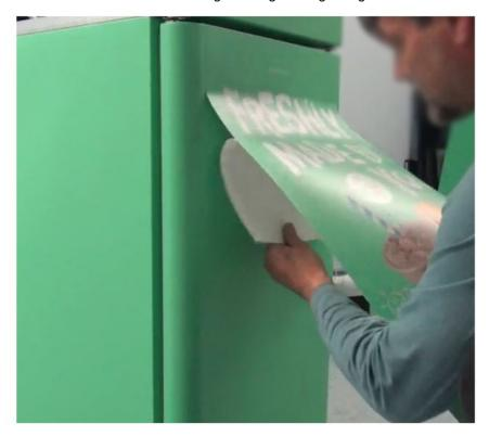
31. Starting at the top of the decal use decal applicator tool to press bubbles out of decal using short strokes moving down towards floor.
