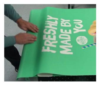
14. Use decal applicator/smoothing tool to press out bubbles along top edge of decal to firmly secure exposed adhesive to panel.
