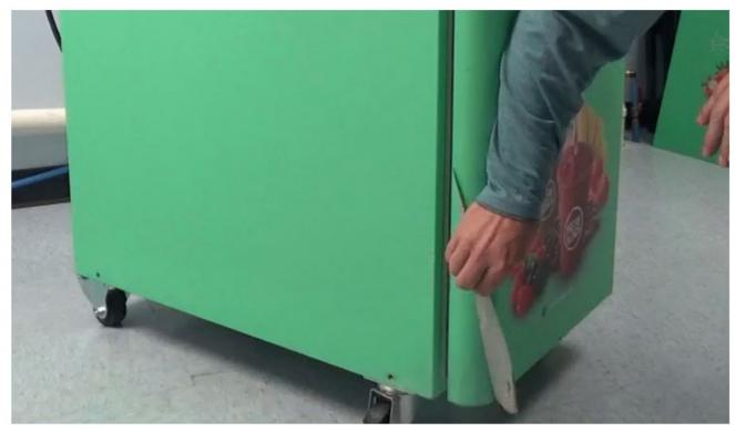
23. Using scissors cut 2-3 inch (5-8cm) slits 6 inches (15cm) apart along loose edge.
