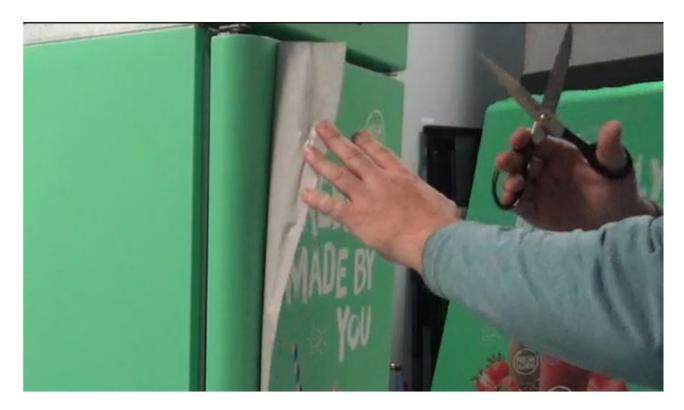
24. Starting at edge with slits, peel away old decal in strips.
