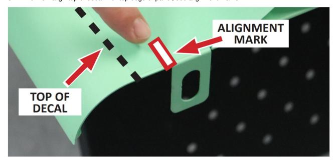
13. Using clean hands start at center of decal and gently press outwards to secure the exposed adhesive back of decal to panel.
