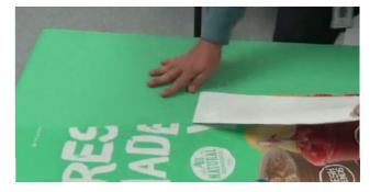
9. Spray panel surface with isopropyl alcohol, scrub surface with clean cloth to remove dirt or adhesive residue. Dry thoroughly with a different clean cloth. Make sure surface is dry and dirt/lint free.
