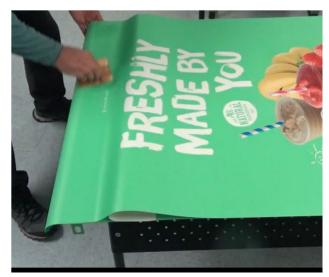
15. With one hand remove remaining backing while guiding the decal onto the panel with other hand.
