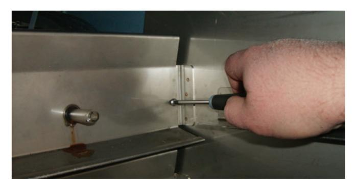
104. Remove four (4) 5/16" head screws that secure the blender belt access cover. Remove the cover.
