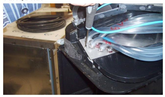
58. Install the divider in between the hoses in the chase.
