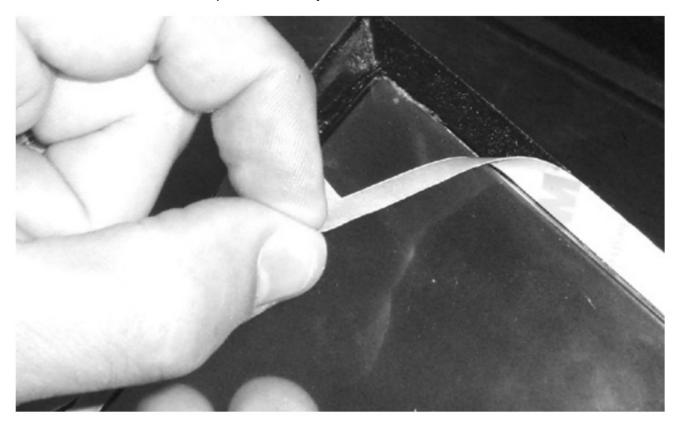
127. Slowly and carefully place overlay into position over the screen. DO NOT press on the adhesive portion of the overlay yet. The overlay should self position itself and fit naturally into the screen opening. DO NOT FORCE the overlay into position.
