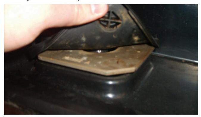
68. Use a 5/64" Allen wrench to loosen the set screw.
