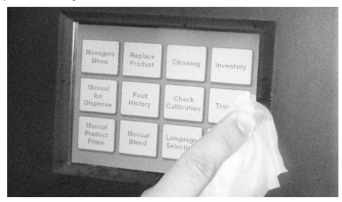
125. With a dry towelette carefully dry the touch screen and beveled surface around screen. Dust and smudges must be removed so there is a clean smooth connection with the touch screen.
