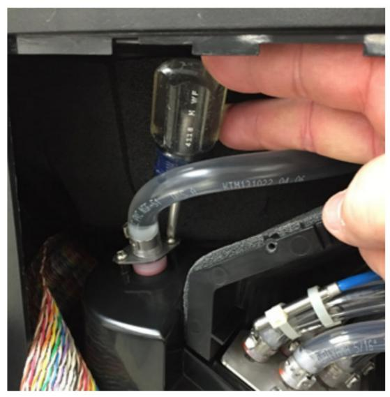
**NOTE**: The product tubing is numbered 1-8. The dispenser head bracket is also numbered 1-8, be sure to these numbers match up when installing.
