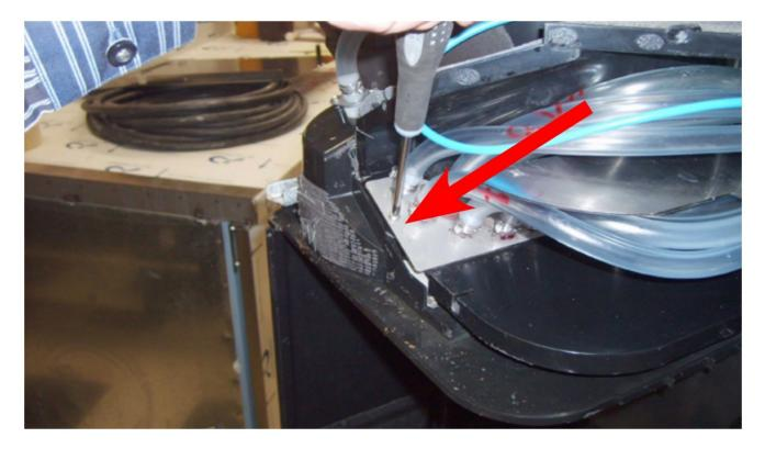
49. Remove the divider from between the hoses in the chase.
