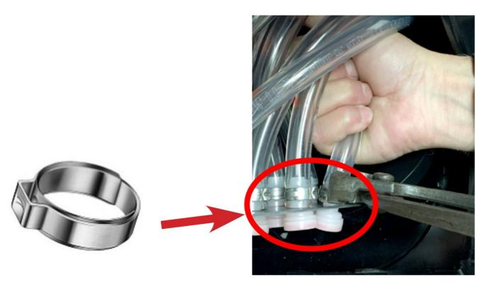
52. Using snips or Oetiker pliers, cut the existing Oetiker clamps that secure the product tubing to the LMS valves. Remove the existing LMS valves and discard.
