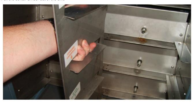
103. Remove two (2) Phillips head screws on the top product bin support plate. Do not remove the product fittings. The plate can sit on top of the support plate below it.
