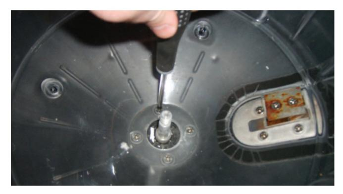
26. Remove the ice bin by lifting it straight up. Be sure not to drop/lose the ice bin lid safety switch actuator rod, check for cracks or broken ice bin. Inspect the ice bin for damage and record notes on the BIM Tune Up Checklist.
