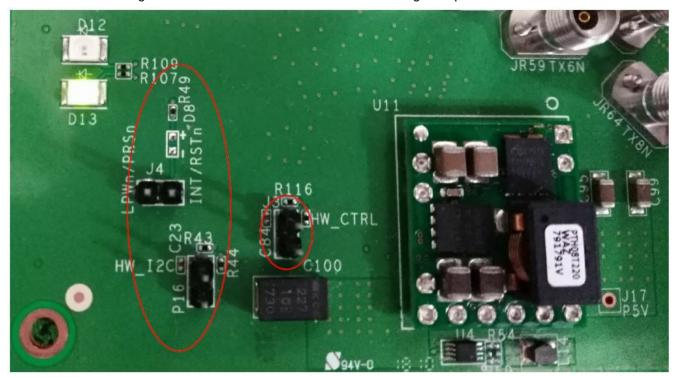
Hardware control signals can be driven through the jumpers. A jumper is placed on J3 HW\_CTRL to be able to control hardware signals from J4. J4 pin headers provides direct access to LPWn/PRSn and RSTn/INT pins of the OSFP connectors
