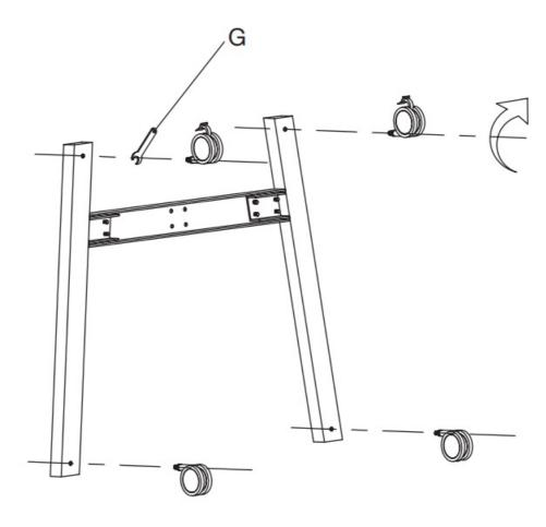
Use the allen wrench to adjust the castors to make the base level, then let the screen levelly
