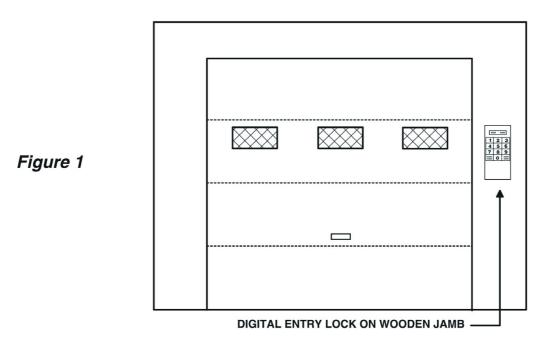
IF YOU ARE MOUNTING YOUR KEYLESS ENTRY SYSTEM TO ALUMINUM SIDING you may find it better to substitute carriage bolts for the mounting screws supplied. Bolts should be long enough to reach into the garage and be secured with lock washers and nuts. IF YOU ARE MOUNTING YOUR KEYLESS ENTRY SYSTEM ONTO BRICK, STONE, OR MORTAR, suitable anchors must be set into the mortar, and the fasteners screwed into these.
