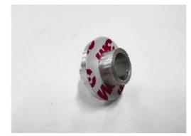
Peel off the backing from the other side of the washer and stick the spacer into the hole in the trim from the inside of the trim. P ress firmly.
