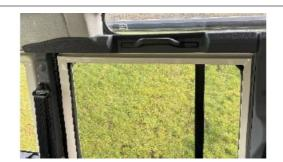
B-Pillar trim is fixed in place with 2 x fir-tree fasteners.
