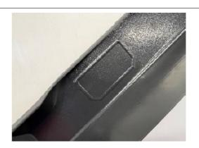
The rear end of the Cant Rail trim tucks behind the front edge of the window trim on 110SW. The front end of the Cant Rail tri m tucks behind the top of the B-pillar trim. Can Rail is fixed in p lace with the grab-handle screws.
