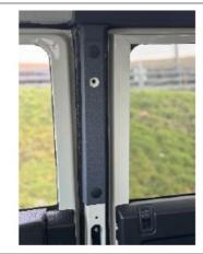
On 110 models slide the seat belt through the gap in one side of the seat belt escutcheon trim and clip it into place.
