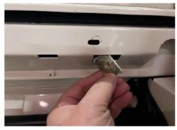
Use the M6 fixings with the spring washer and flat washer thro ugh the rear seat bracket uprights to secure the panel. Yes. Th ey're awkward and fiddly to get started! Blame Land Rover. A p en-style magnet can be useful for holding the threaded plates f or this task.
