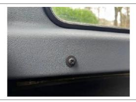
The front lower corner of 90 & 110 panels is secured with fir-tre e fasteners. Note that if you're converting a 90 Hardtop (van), t he Hardtop models are not fitted with the corresponding corner bracket that the fir tree fits into. The Land Rover part number f or the bracket fitted to factory Station Wagon models is MXC32 76 or create your own from a bent piece of steel.
