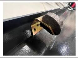
The aluminum tubular spacers attach to the back of the large h oles running across the bottom of the panel.
