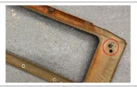
The threaded lower fixing plates slide into the rectangular open ings in the bottom of the body
