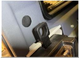
The Cant Rail has witness marks on the reverse of the RH pan el that will need cutting out to provide the mounting hole for the alarm sensor (when fitted).
