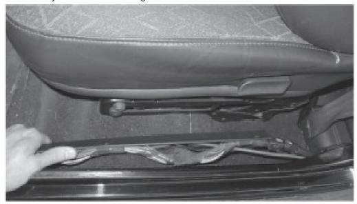
Step 6 – Use a Phillips screw driver to remove the three clips holding the factory wire harness under the door threshold on the driver side.
