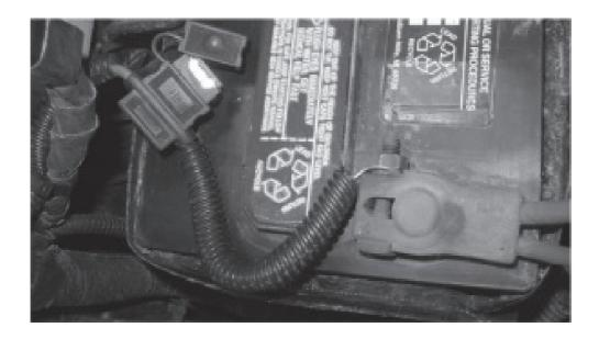
Step 15 – Ground amplifier to chassis of the vehicle; connect the terminal provided to the 10ga black wire from the furnished wiring harness. A good ground is as important as the power connection. The ground should be as short as possible and the contact point should be free of paint and debris.
