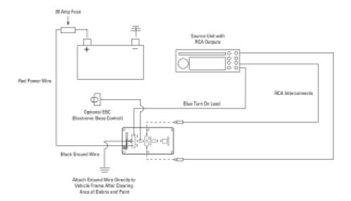
Step 18 – Plug power wire harness into amplifier pre-amp.
