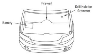
Step 11 – Route 10ga red power wire through the grommet into the engine compartment.
