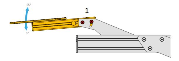
1. Loosen the screws marked in red to tilt the desk.
