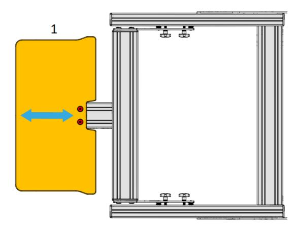
1. Loosen the screws marked in red to change the distance of the desk.
