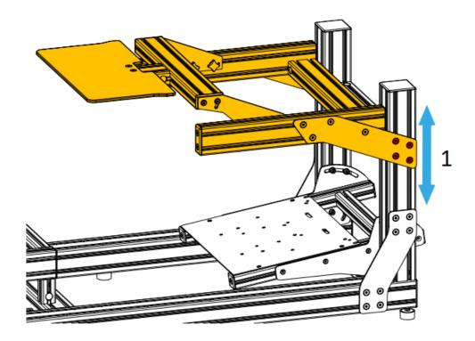
1. Loosen the red marked bolts on each side to adjust the height.
