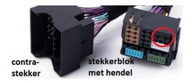
Remove this optical plug by pressing the tab and gently pulling the plug out of the power strip with the
