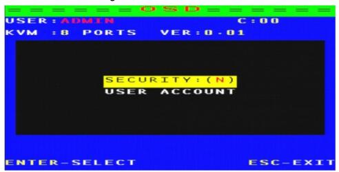
When you press F7 into the user settings, the screen shown in Figure 4, SECURIY: Y represents that need the password to enter, N on behalf of don't need the password to enter, press the "," into the user account, Press "enter" to into, enter the screen as Figure 5
