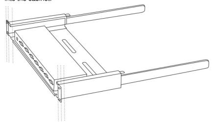
**Step 2:** At the front side of the cabinet, insert the display terminal and the big tray into the support arm of the small tray, and then fix the cabinet screws.
