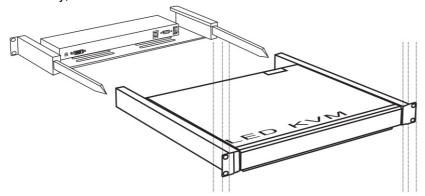
Step 3: Connect the KVM module and the display terminal via the DVI cable
