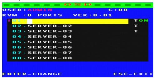
**Note:** You can change the name of the host as you like, use the keyboard up and down key to control, when you need to change the host name, press the enter on keyboard can be changed
